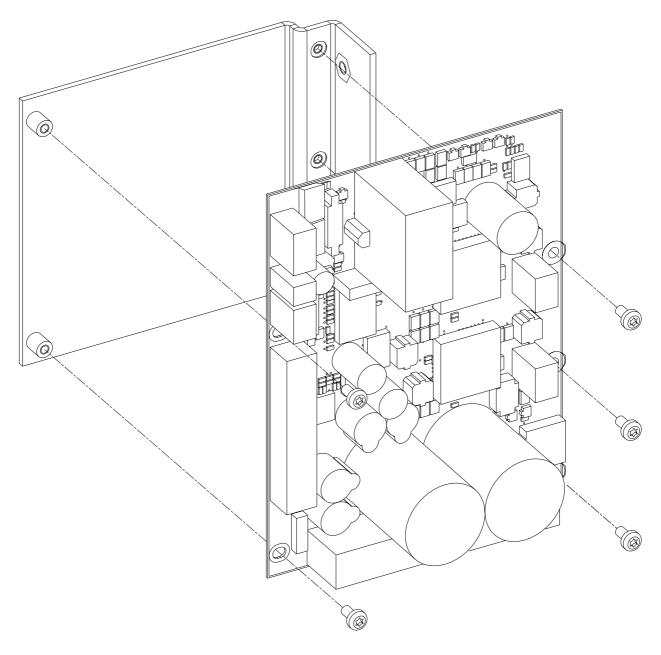
The driver board and its attachment plate come as an assembled spare part.
