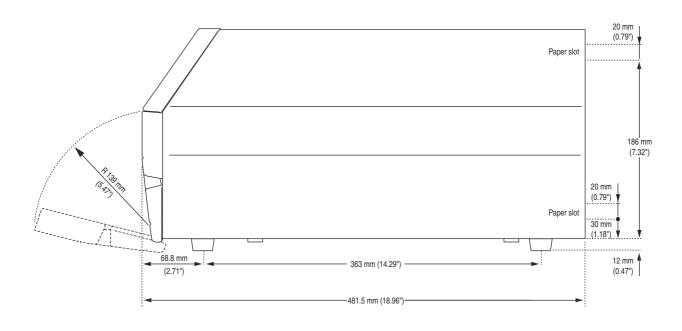
An optional paper cutter increases the printer's total length by 28 mm (1.1 inches). At least 90 mm (3.5 inches) of free space behind the printer is required for the connectors, and for inserting and removing a memory card.
