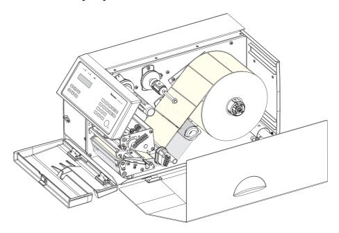
The liner takeup unit can accommodate the liner from a full roll of labels.
