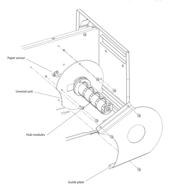
The media supply hub package can be dismantled by removing the #T20 Torx screw at the end of the shaft. Inside the outermost hub module, there is a spring that presses the hub package towards a felt pad in order to break the rotation. Else, the momentum of a large and heavy media roll might cause excessive media to be unwound when the printing is stopped. The brake torque should be 70 ±20 Nmm (see Appendix C).
