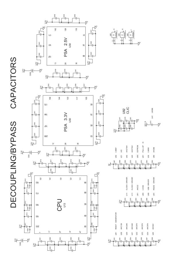
1-971630-26 CPU Board; Bypass/Decoupling (Schematics #9)
