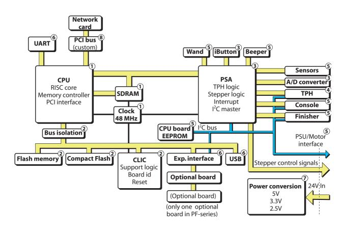
1-971630-26 CPU board; Block Diagram (numbers refer to schematics in Chapter 15.7)
