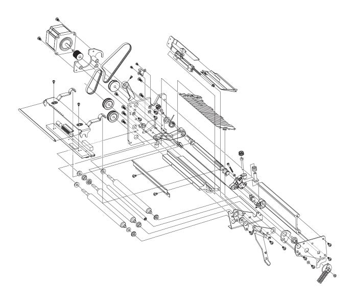
The parts of the print mechanism fitted inside the electronics compartment in an EasyCoder PX4i printer are illustrated below.
