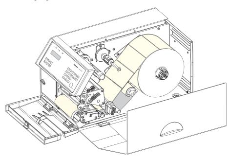
The batch takeup unit can accommodate approximately 1/4 to 1/3 of a full label roll depending on media thickness.
