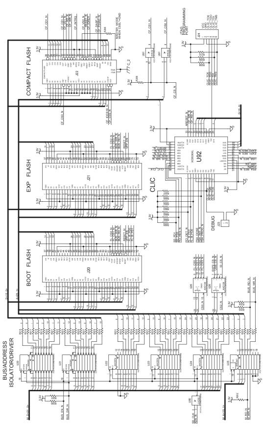
1-971630-26 CPU Board; Flash Interfaces (Schematics #2)
