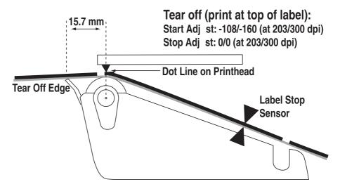
When using peel-off operation, the labels would drop from the liner and get stuck on for example the desk if you use the default Start Adjust value 0. Use a Stop Adjust value of around -40/-60 (= 5.5 mm/0.22 inches) instead: that is, after the printing is completed 5.5 mm/0.22 inches less of media feed than normal will be performed. However, if you still want to print from the top of the label, you must compensate by a Start Adjust value of around -80/-115 (= 10.0 mm/0.39 inches).
