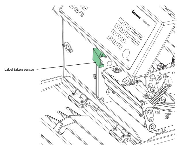
The photoelectric sensor emits a narrow beam of light, which will be reflected back to the sensor by any label, ticket, tag, piece of strip, or liner, that has not been removed from the outfeed area.
