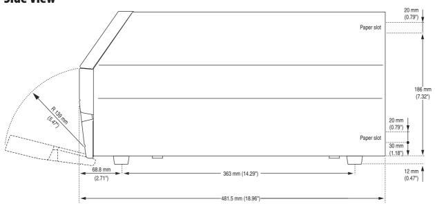
An optional paper cutter increases the printer's total length by 28 mm (1.1 inches). At least 90 mm (3.5 inches) of free space behind the printer is required for the connectors, and for inserting and removing a memory card.
