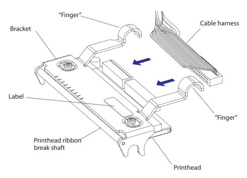
Illustration shows the printhead of an EasyCoder PX4i.
