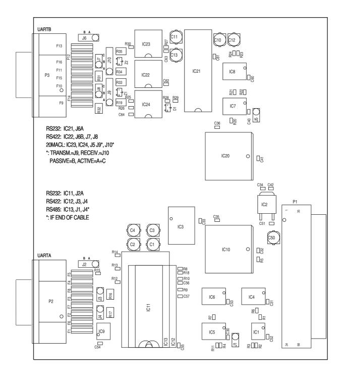
1-971642-26 Double Serial Interface Board; Component side
