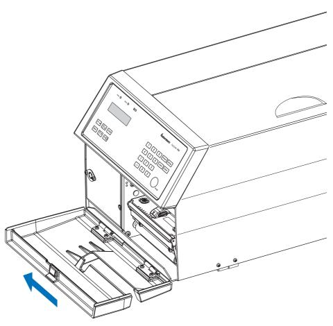
The front hatch can be removed by pushing it to the left when open (illustration shows an EasyCoder PX4i).
