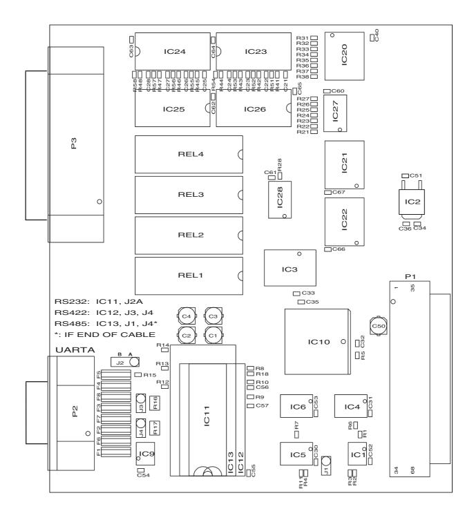
1-971643-26 Serial/Industrial Interface Board; Component side
