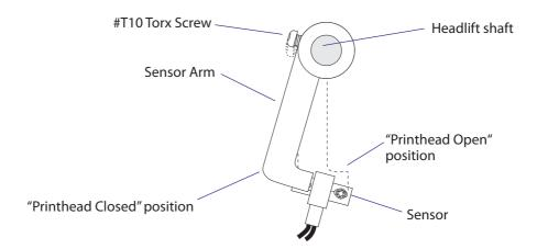
In Fingerprint, run this program which assists you in adjusting the headlift sensor arm:
