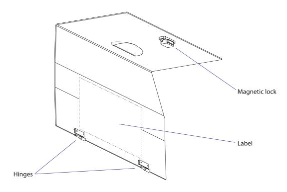
Illustration shows the right-hand door of an EasyCoder PX4i. The door of the EasyCoder PX6i has a wider top part.
