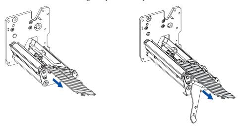
When cleaning the guide plates, use a soft cloth moistened with isopropyl alcohol. Do not use any other type of chemicals. Blow the sensors free from dust.
