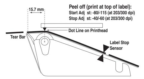
A special case is tickets with black marks. It is recommended to place the black mark adjacent to the perforation or the intended tear-off line. If the black mark is placed further down the media, this must be compensated for by a negative Stop Adjust setting.
