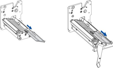
• To remove the lower guide plate, disengage the snap-lock (accessible through a slot in the lower gable) using for example a screwdriver and lift the outer end of the guide plate. Then pull it out.
