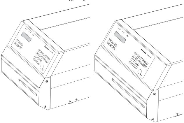
The cutter is intended to cut through continuous non-adhesive paper strip or through the liner between labels. It must not be used to cut through any kind of adhesive or other soft material, that may stick to the cutting parts and render the cutter inoperable or even damage the electric motor.
